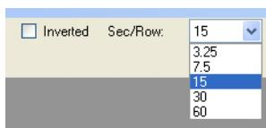
To invert the ECG signal, check or uncheck the **Inverted** box.
