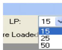
To adjust the Low Pass filter, click on the drop-down box labeled **LP**. This filter will allow you to reduce muscle noise and electrical artifact.
