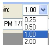
To change the amplitude of the displayed signal, click on the Gain field and select a different size from the list.
