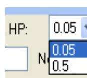
To adjust the High Pass filter, click on the drop-down box labeled HP. This filter will allow you to reduce baseline wander.
