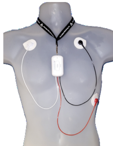
3-lead adapter with lanyard placement. Electrodes required.
